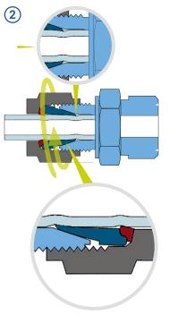
For screw connections up to 4 mm, only one 3/4 turn from the hand-tight position is permissible..
