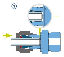
• Hold the fitting body firmly and mark the position of the union nut. Complete the clamping using a wrench by turning the nut a 1 1/4 turn (Fig. 2). The connection is now correctly mounted.
